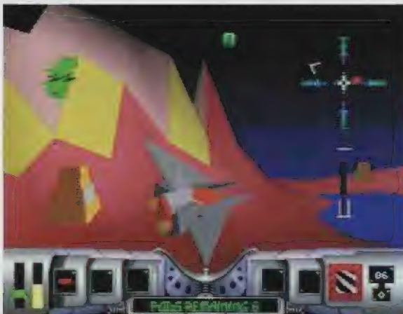
Cybermorph makes full use of the Jaguar's built-in Z-buffering, which allows 3D objects to be easily displayed in relation to one another – sitting on top of or even intersecting other polygons
